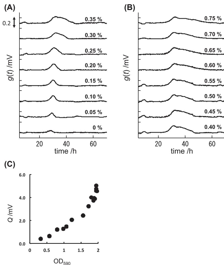
FIG. 4. Growth thermograms (A, B) of *C. beijerinckii* generated for cultures with various glucose concentrations. *C. beijerinckii* was grown with between 0% and 0.75% glucose. (A) From the bottom, 0%, 0.05%, 0.10%, 0.15%, 0.20%, 0.25%, 0.3% and 0.35% glucose. (B) From the bottom, 0.40%, 0.45%, 0.50%, 0.55%, 0.60%, 0.65%, 0.70% and 0.75% glucose. (C) Plot of  $Q$  versus OD.
