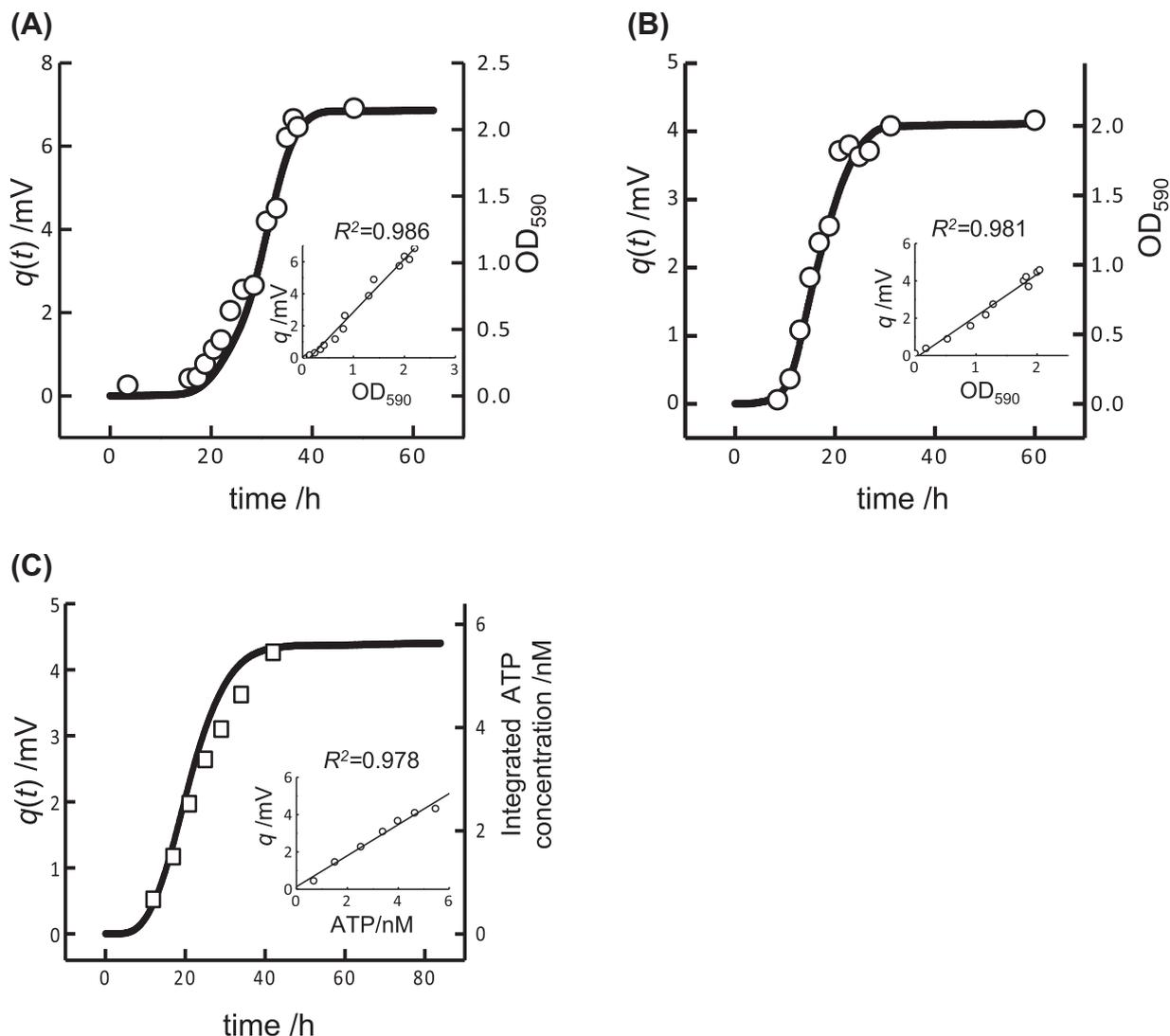
FIG. 3. Time courses of heat evolution by *C. acetobutylicum* (A), *C. beijerinckii* (B), and *C. cellulovorans* (C). *C. acetobutylicum* (A) and *C. beijerinckii* (B) were grown with 5% glucose. *C. cellulovorans* (C) was grown with 0.5% cellobiose. The  $q(t)$  of each strain was calculated from  $g(t)$  obtained using the multiplex isothermal calorimeter (line). Circles and squares indicate optical density and integrated ATP concentration, respectively.
